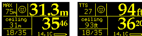
Direct ceiling display: deco ceiling limit with smiley depth guide.
