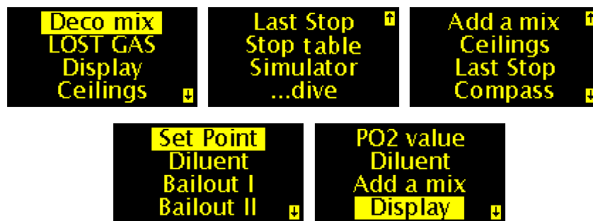
Sample OC and CCR underwater menu items.
