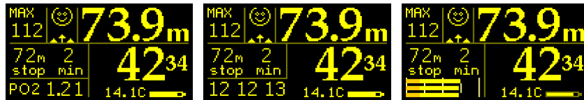
Three ways to display PO2 information: Hi cell, 3 cells or bars (1.2 shown). These are selected via the Config setting, and the UW display menu item.
