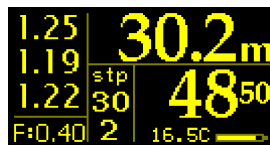
This screen is available during the dive with Screen scroll taps. The data shown is 3 cells, with expected flush reading shown.
