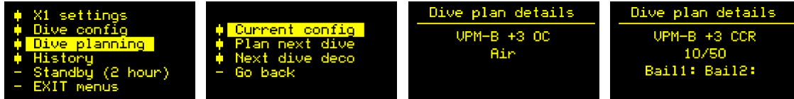
Two samples of dive plans: OC air dive, CCR dive with 10/50 diluent and no bailouts.
