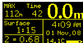
Surface display with scrolling PO2 cell readings (cell #2 shown).
